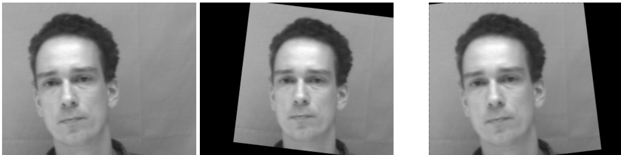
Figure 14: Sequence of images to exemplify the processing steps of a simple video-conference system. The left image is a newly acquired video frame. The middle image is the most similar normalized example image found in the database. The pose parameters of the new image with respect to the reference example are estimated and transmitted together with the index number for the example. On the receiver side the stored normalized example is transformed towards the pose of the new image on the sender side (right image).
